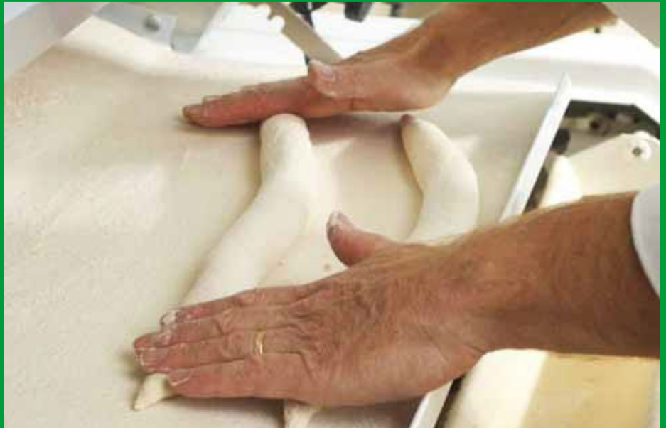
Rolled pieces of dough at the output of the moulder
