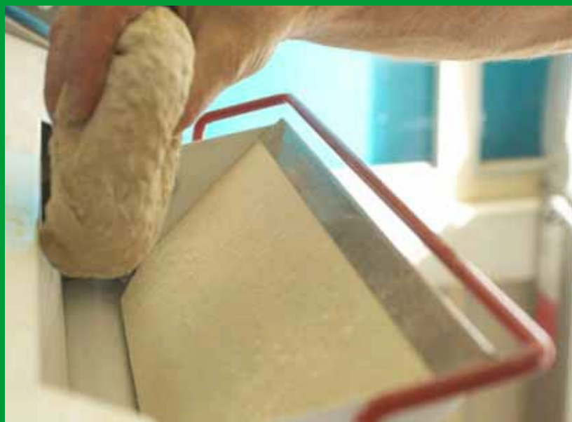
Simple insertion of the dough piece in the Major moulder
